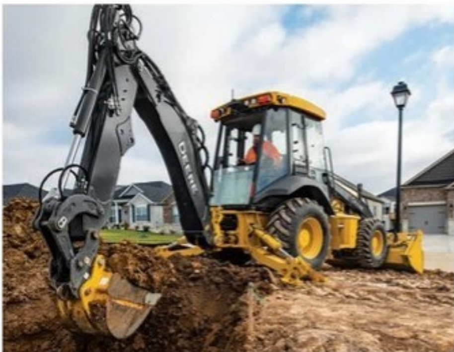
John Deere's 310 L model backhoe loader is equipped with standard length stabilisers.
