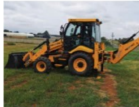
The side-shift backhoe is suited to trenching in tight spaces.
